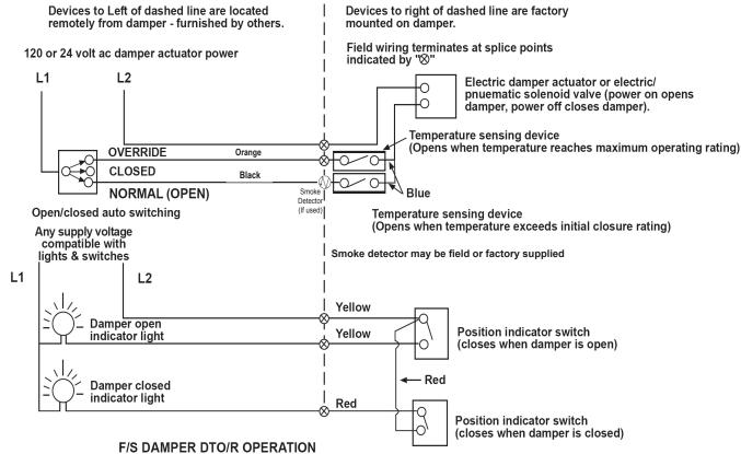
Switch is in Normal (Open) Position damper motor is energized until thermostat senses temperture above initial closure rating. Above termperature closure rating, the damper motor is de-energized and damper closes.
